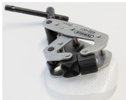
Figure 2: Induction of occlusion in steel needles (left) and soft cannula (right).
